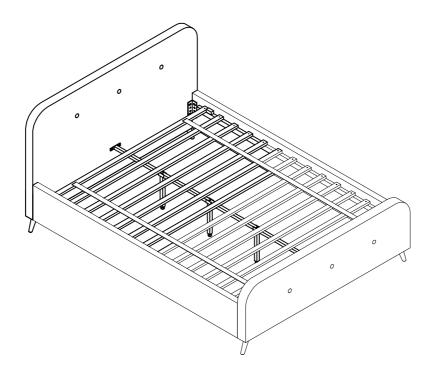
Do not tighten bolts until completely assembled.
